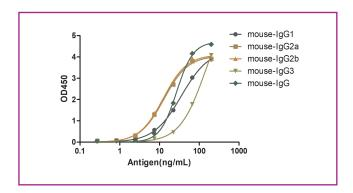
A titer ELISA of mouse IgG. The plate was coated with different amounts of mouse IgG or different isotope of mouse IgG. 1:10000 dilution of Anti-Mouse IgG(Fc $\gamma$  Fragment specific), AlpHcAbs® Goat antibody was used as the primary antibody. An HRP conjugated anti-Goat IgG as the secondary antibody.
